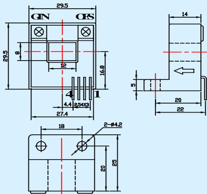
Elucidation: 1:+5V 2: 0V(GND) 3: V<sub>OUT</sub> 4:ref (2.5V) OFS:Zero adjustment GIN:Gain adjustment
