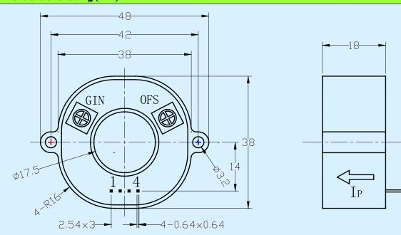
Elucidation: 1:+15V 2:-15V 3:V<sub>OUT</sub> 4:0V(GND) OFS:Zero adjustment GIN:Gain adjustment
