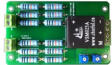
Closed loop voltage sensor based on the principle of Hall-effect. It can be used for measuring alternating, direct, pulsed and mixed voltage
