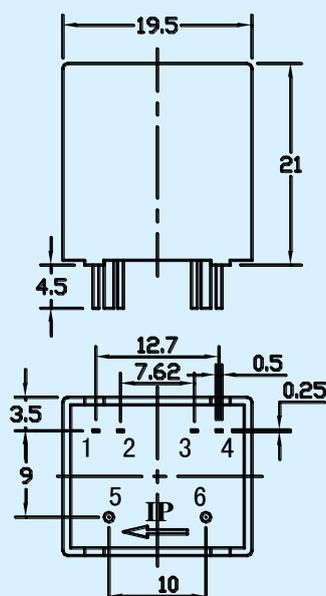
Elucidation: 1:V<sub>OUT</sub> 2:+15V 3:-15V 4:GND 5:-Input 6:+Input
