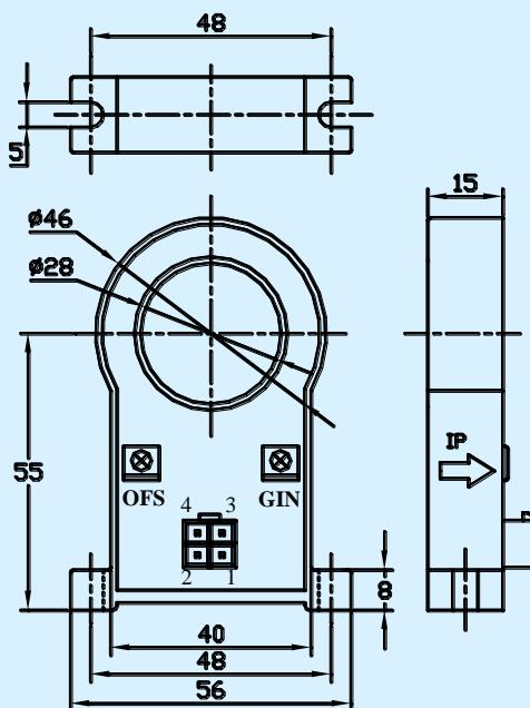
Elucidation: 1:0V 2:-15V 3:V<sub>OUT</sub> 4:+15V    OFS:Zero adjustment    GIN:Gain adjustment
