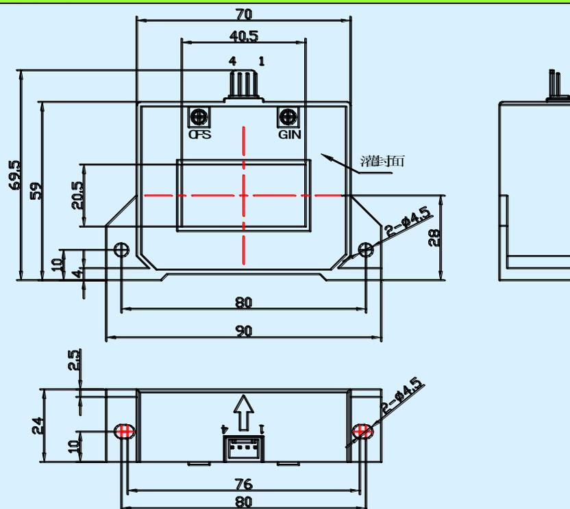
Elucidation: 1: +15V 2: -15V 3:  $V_{OUT}$  4: 0V(GND) OFS: Zero adjustment GIN: Gain adjustment
