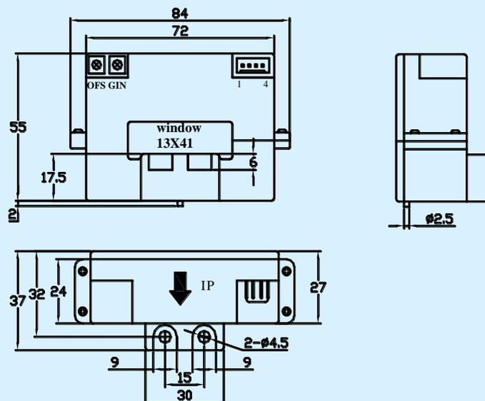
Elucidation: 1:+15V 2:-15V 3:  $V_{OUT}$  4:0V(GND) OFS:Zero adjustment GIN:Gain adjustment
