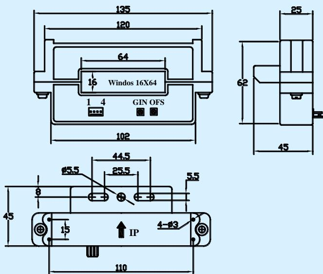
Elucidation: 1: +15V 2: -15V 3: V<sub>OUT</sub> 4: 0V(GND) OFS: Zero adjustment GIN: Gain adjustment
